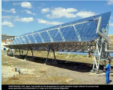
Line focus and flexible joints
